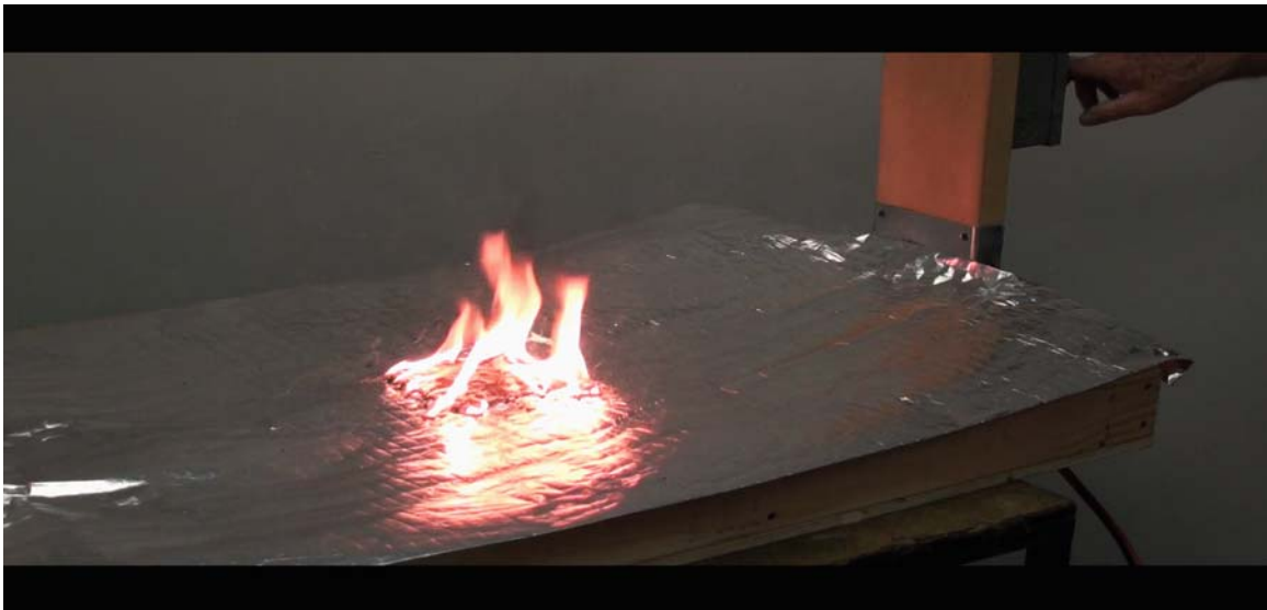
PHOTO #1 (from a previous study) Radiant Barrier Material in Flames After Being Energized by a 20 Amp Circuit
