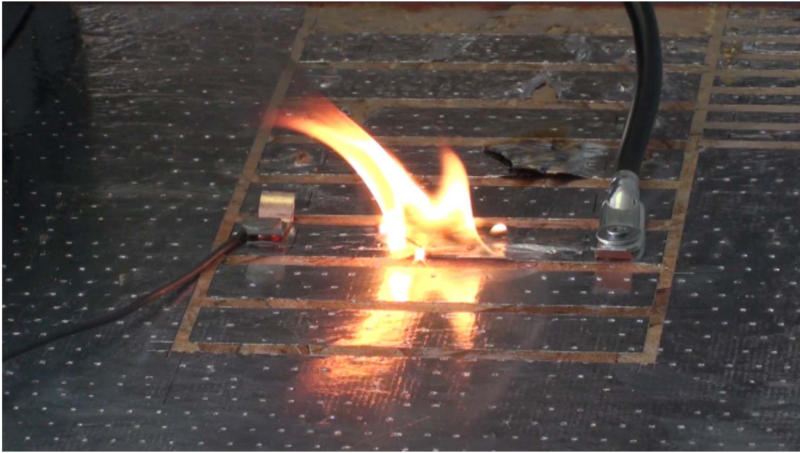
PHOTO #8 One Inch Wide Test Strip Energized With Current of Approximately 50 Amps
