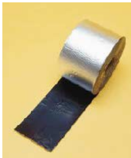
Figure 3. Since foil-topped flashings like Peel'N'Stick from Polyguard Products can be left exposed to the weather for a longer period than polyethylene-topped flashings, they are a good choice when siding installation may be delayed.
