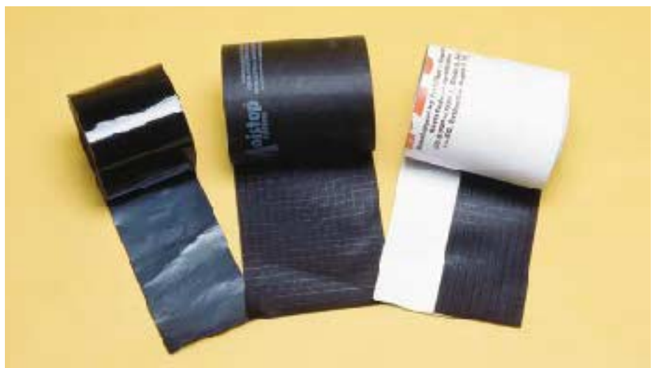
Figure 6. Not all flexible flashings are self-adhering. Future Flash from MFM Building Products (left) and Moistop from Fortifiber (center) are nonstick flashings that are installed with fasteners. Fortifiber's Moistop E-Z Seal (right) is similar to regular Moistop, but includes a 3-inch-wide adhesive band along one side of the flashing.
